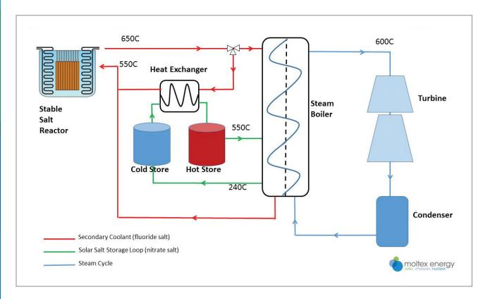
But the Stable Salt Reactor produces its heat at just the right temperature for this heat storage technology, around 600°C.
